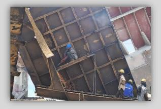
Ship recycling today heavily depends on labor-intensive methods with considerable safety and health risks like direct injuries and long-term health effects. Workers can be exposed to toxic fumes while cutting metal coated with paint, leading to potential occupational diseases. Fire and explosions as well as falling objects or falling from height are also common risks.
